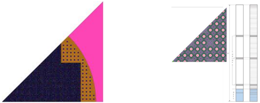
Figure 3: Radial (left) and axial (right) reflector benchmark configurations
