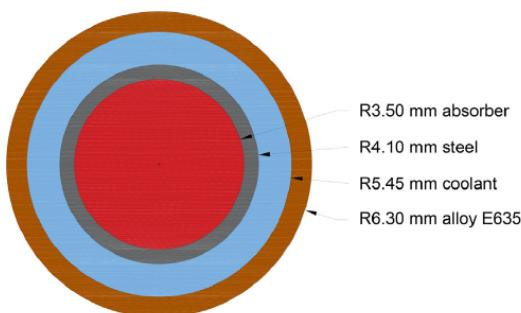
**Figure 13: Khmelnitsky-2 guide tube with control rod cell [7]**
