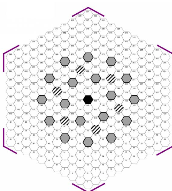
**Figure 4: Khmelnitsky-2 fuel assembly type 398GO [7]**
