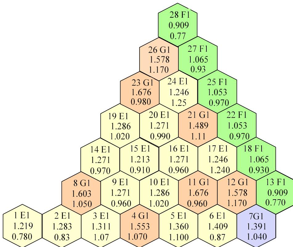
**Figure 32: Core loading for cycle 1 – Kozloduy-6 [5]**
