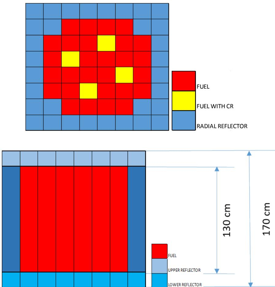
Figure 20 : PWR minicore radial and axial mapping
