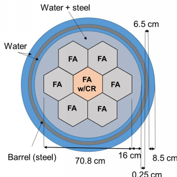
Figure 16 : Mini-core configuration based on Kozloduy-6 [8]
