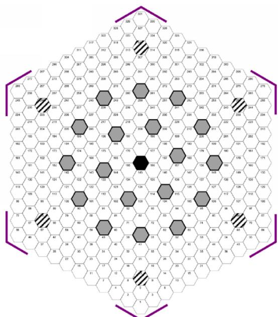
**Figure 3: Khmelnitsky-2 fuel assembly type 439GT [7]**
