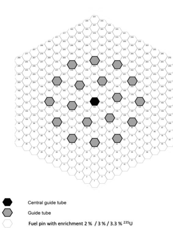
**Figure 1: Kozloduy-6 fuel assembly type UOX 2%, 3%, 3.3% and 4.4%**
