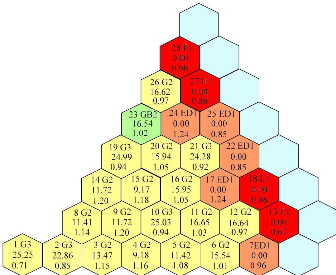
Figure 33: Core loading for cycle 6 – Kozloduy-6 [5]
