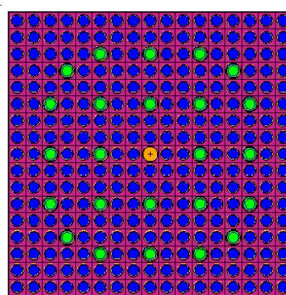
**Figure 21 : UOX 3.7% 2D assembly layout**
