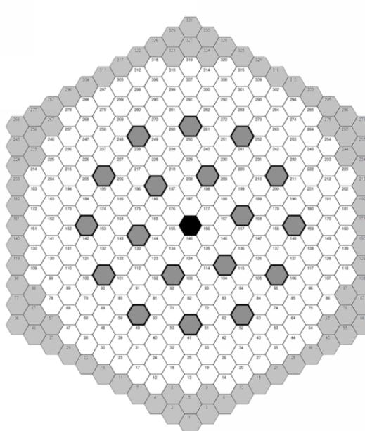
**Figure 6: Kozloduy-6 profiled fuel assembly 2D assembly layout**
