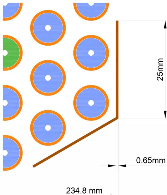
**Figure 15: Corner stiffener geometry [7]**
