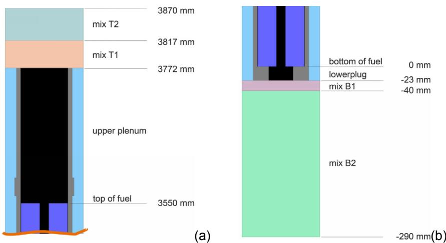
**Figure 19: Axial layout of the fuel pin model Khmelnitsky-2 [7] – upper (a) and lower (b)**
