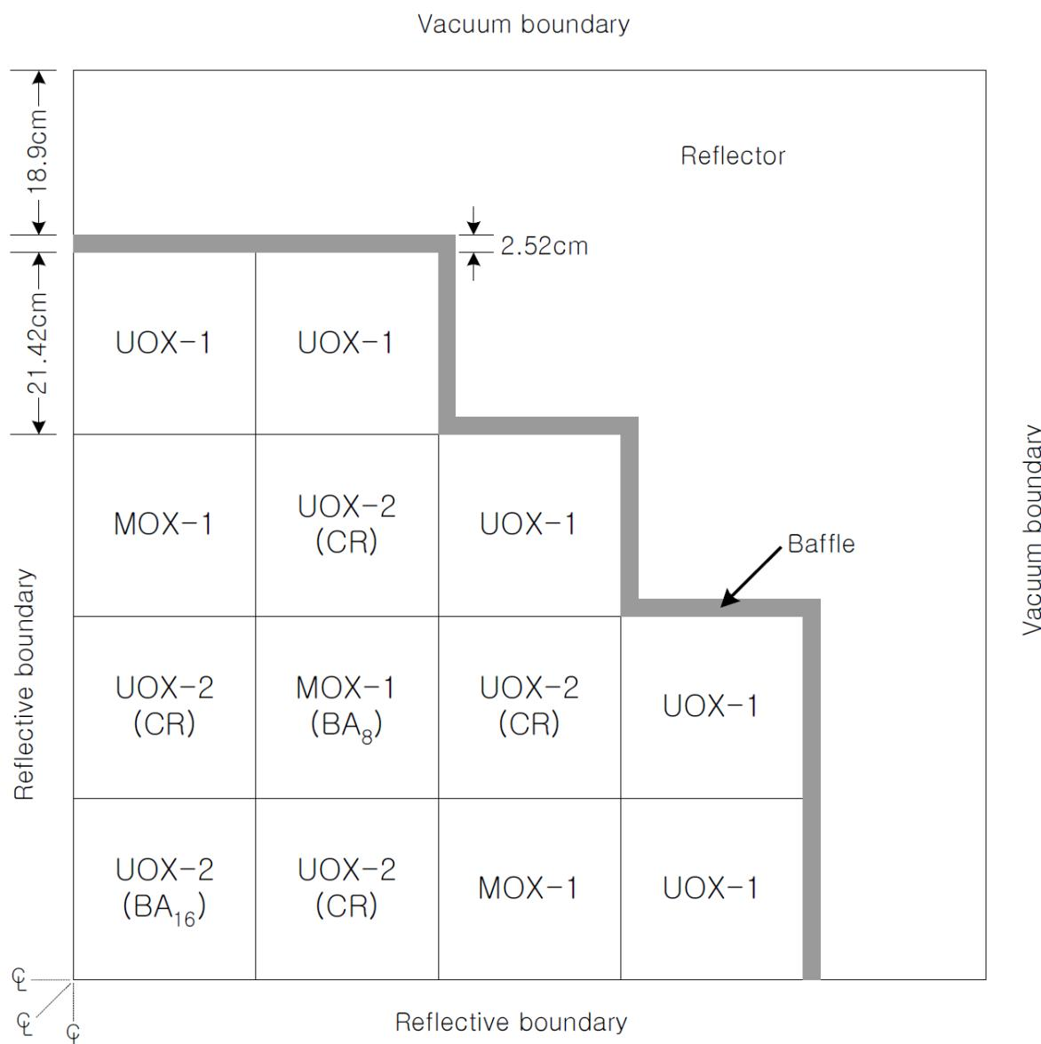
**Figure 30: KAIST 2D core and radial reflector configuration [9]**
