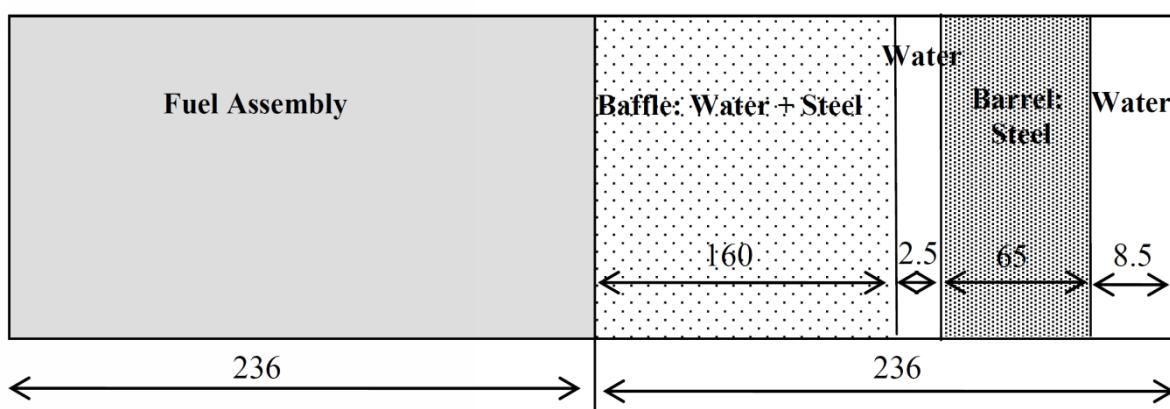
**Figure 17: Kozloduy-6 mini-core radial reflector cross-section [2]**
