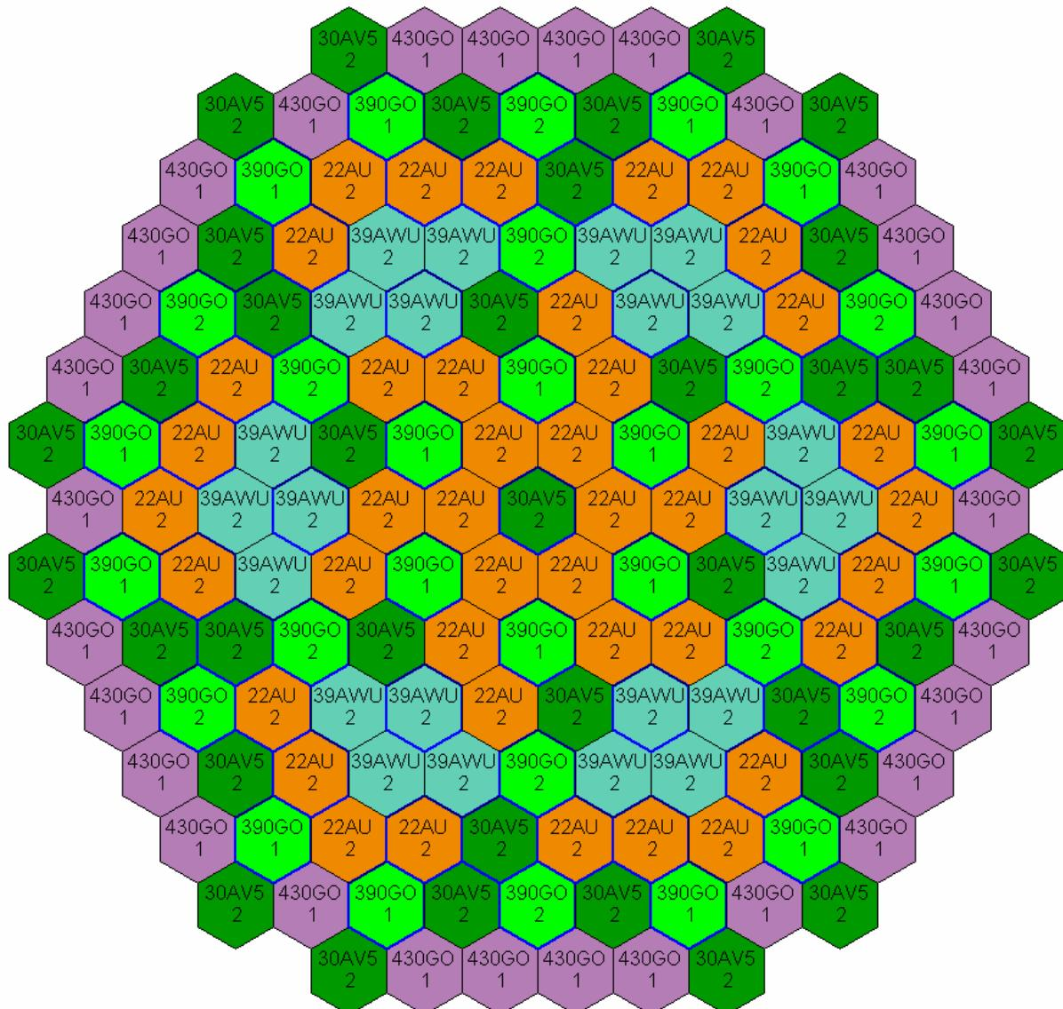
Figure 36: Core loading for cycle 2 – Khmelnitsky-2 [6]
