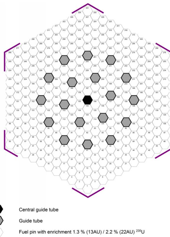
**Figure 2: Khmelnitsky-2 fuel assembly type 13AU and 22AU [7]**
