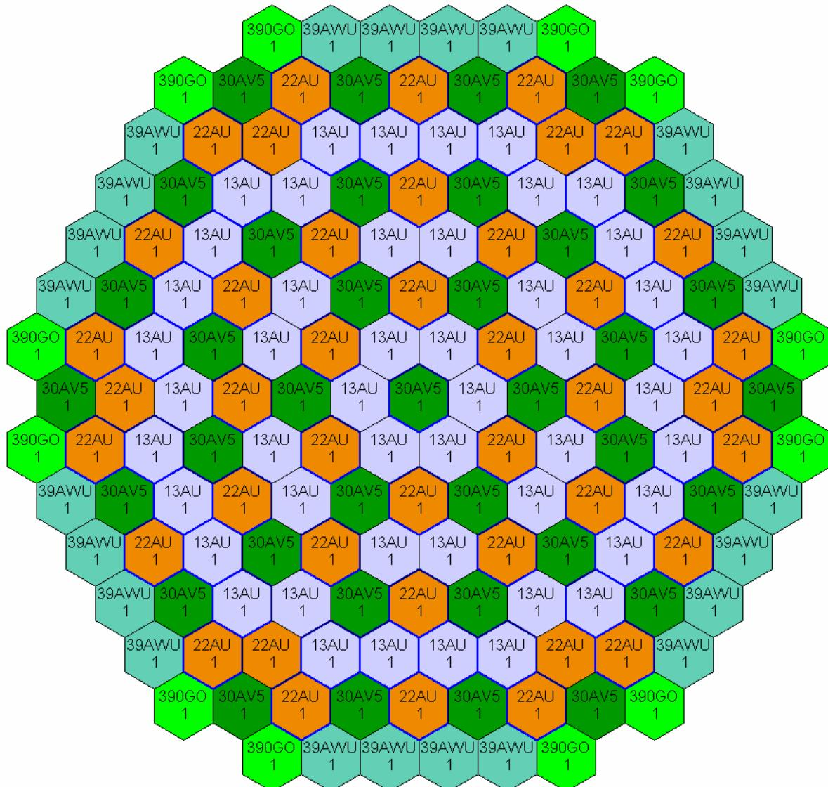
Figure 35: Core loading for cycle 1 – Khmelnistky-2 [6]
