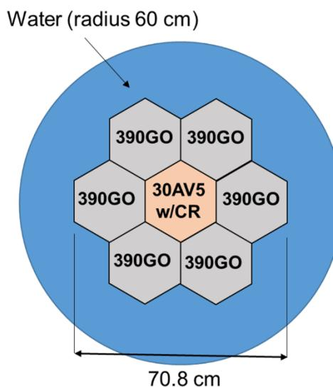
**Figure 18: Mini-core configuration based on Khmelnitsky-2 [8]**
