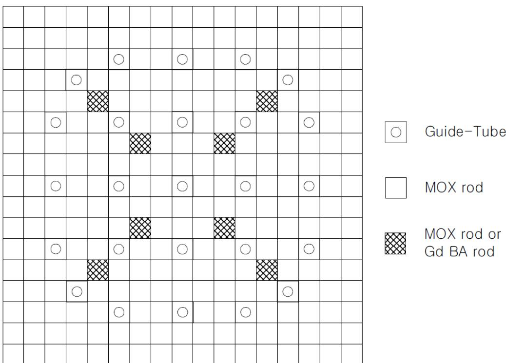
**Figure 27: KAIST fuel assembly 2D assembly layout – MOX without zoning [10]**
