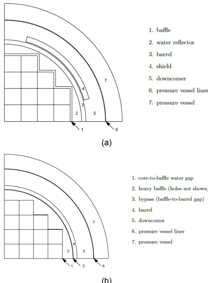
**Figure 31 : Reflector configurations proposed by CEA:**
